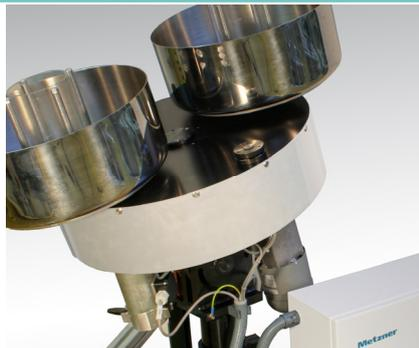
The Metzner CPC 400 is an automatic cable coiler for flexible cables and lines up to 15mm in diameter. The device is highly productive with either the two or four alternately driven coiling pots: While the already coiled cable is being removed from one pot, the cable processing machine already fills the next pot.
