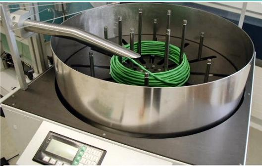
The Metzner CRC 750 cable coiler coils cables of even large diameters fully synchronously with the work cycle of the cable processing machine.
