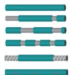
Cutting of cables and strands Stripping with partial and full pull-off Window stripping Extremely long pull-offs in multiple stages Cutting and stripping of teflon cables Printing and marking
