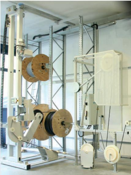
**Cable rack with automated cable reel handling**
