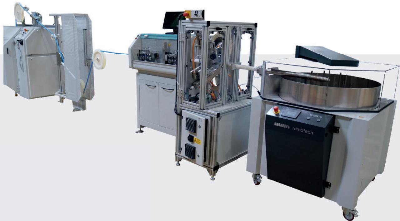
For downstream processes cables often need to be cleaned and either talcum used during the cable manufacturing process or surface dirt has to be removed. This job is successfully mastered by the Metzner inline cable cleaning station.
