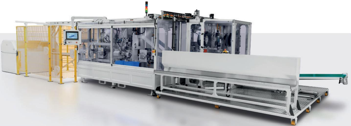
Due to their unique design, high-frequency coaxial cables call for very different processes compared to standard coaxial cables. Metzner developed the required process stations for those cables and integrated them into an automatic processing machine for cable preparation results shown below.
