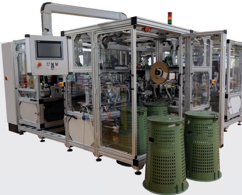
The customer produces wire harnesses that are used in dashboards. For this, cables have to be cut to length, stripped and crimped. In addition, a shrink hose is pulled-over. Up to 4 cables are welded together.
