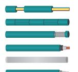
Jacket stripping of multi conductor cables
