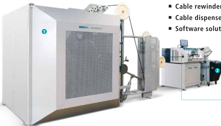
AM 5800 expanded into a production line with 1) electric pay-off for large cable drums and 2) ring coiler
